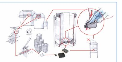
marine litter in coastal cities. URBASER has developed a very simple and circular solution: a small device made with the rubber part of old containers is placed at the bottom of the bin and firmly holds the plastic bag. The production process is simple and is currently being done by a social association. This device named "antivolabossa" (no-blowing bag) was cited in a United Nations publication as one of the top 25 innovative actions to reduce marine litter.
