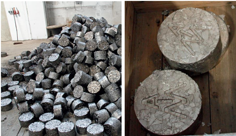
Figure 4.20. Examples of briquetted aluminium swarf (Source: ATM, 2013)
