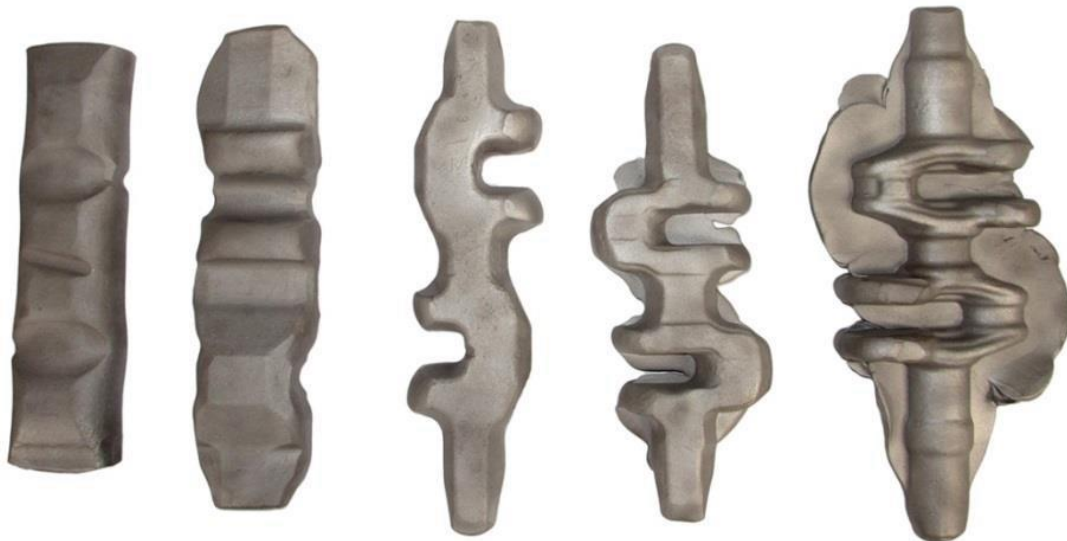
Figure 4.25. Workpiece stages during the five forging steps that are needed for the finished crankshaft. The fourth step takes place with the multidirectional tool (IPH-Hannover, 2014)
