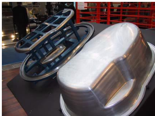
Figure 4.14. Supporting tool in the background of the mould for a bathtub (Nordic Industrial Fund, 2003)
