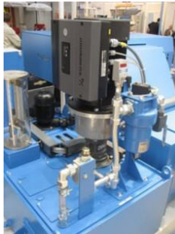
Figure 4.8. Platform for high pressure cooling lubricant supply (Mayfran GmbH)
