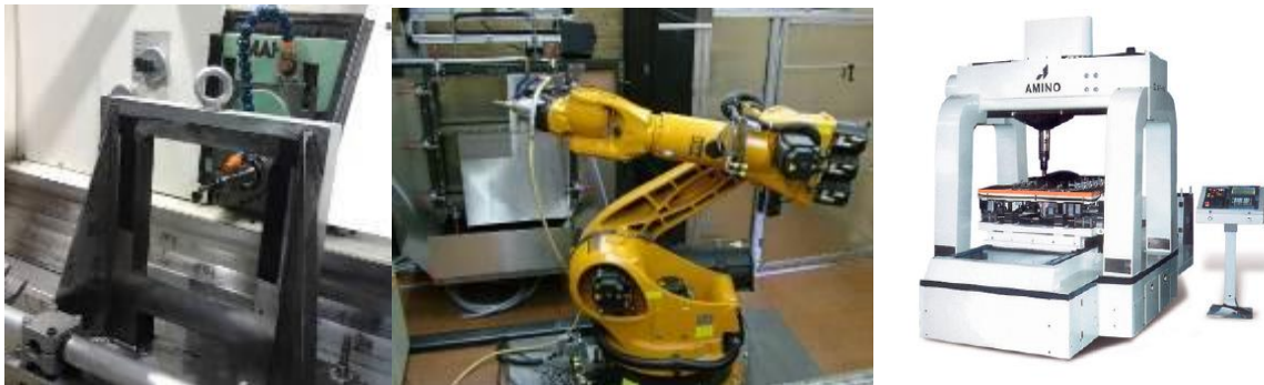
Figure 4.12. Platforms used for ISF, from left to right: CNC milling machine, industrial robot, dedicated machine (Aminio, 2015)
