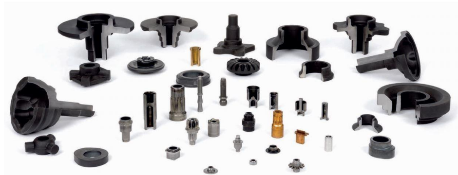
Figure 4.23. Examples of components that can benefit from “flash free” and multidirectional forging (Hatebur, 2015)
