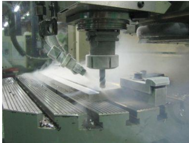
Figure 4.2. Cryogenic cooling for a drilling process (Toolingandproduction, 2017)
