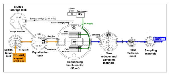
Figure 6.19: Layout of the biological treatment plant of the Hotel Schindelbruch, based on a scheme provided by Mall GmbH, it is designed for 300 person equivalents
